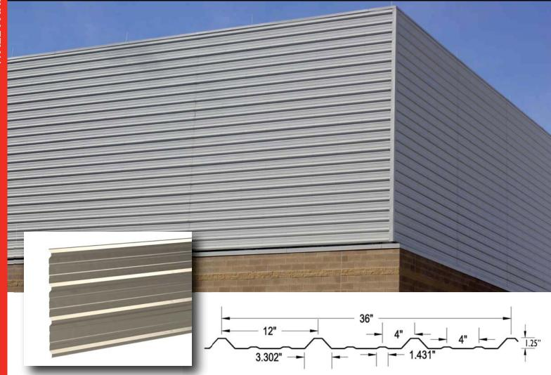
**R PANEL WPRP** is an exposed fastener panel utilized for wall and roof applications. It has an 1-1/4" rib height at 12" o.c. and 36" of panel coverage with a purlin bearing leg.
