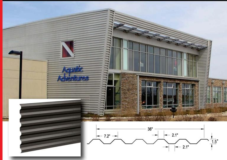
**7.2 PANEL WP72** symmetrical design allows for versatility in applications while providing a clean industrial look. It is an exposed fastener panel utilized for wall and roof applications. It has a 1-1/2" rib height at 7.2" o.c. and 36" of panel coverage with a purlin bearing leg.
