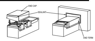
Apply butyl sealant to concealed face for both end caps and end terms. Install end terms and end caps by hooking front face on cleat and pushing down until coping is engaged on both sides of the cleat. Once in place a pop rivet must be installed on inside face of end cap and end term approximately 12" from the wall end.
