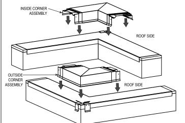
Install miter by engaging top hem of miter to cleat, then press downward to engage bottom. Ensure that both hems are fully engaged before proceeding. Slide a splice plate on either side of miter until approximately half of the splice plate is left exposed. Crimp miter once it is fully engaged and both splice plates positioned correctly.
