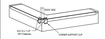
Install two corner support clips at all corners approximately 3" from corner. Secure clips using #14-13 x 1-1/2" DP1 in all pre-punched holes.
