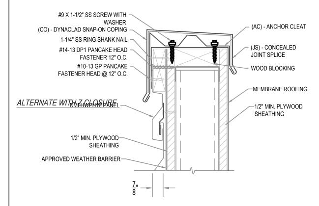
MAXIMUM PANEL ATTACHMENT FASTENER SPACING IS 24" O.C. ALL FASTENERS TO PENETRATE WOOD 3/4" MIN. AND METAL FRAMING 1/2" MIN.
