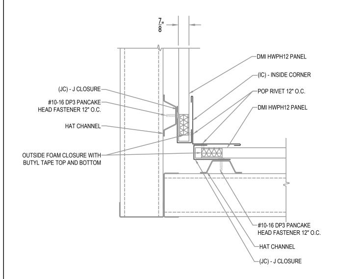
MAXIMUM PANEL ATTACHMENT FASTENER SPACING IS 24" O.C. ALL FASTENERS TO PENETRATE WOOD 3/4" MIN. AND METAL FRAMING 1/2" MIN.
