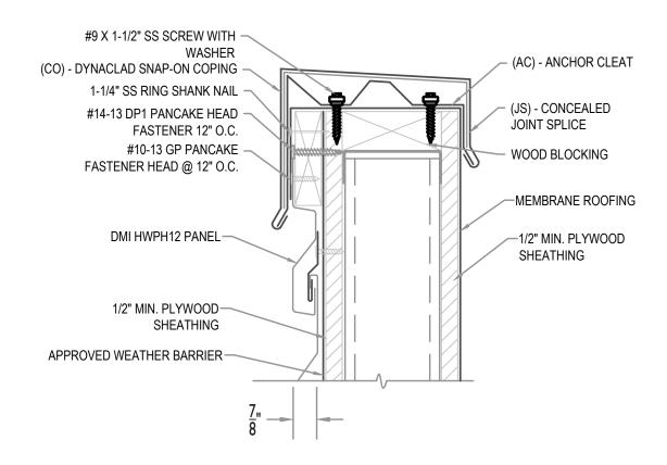
MAXIMUM PANEL ATTACHMENT FASTENER SPACING IS 24" O.C. ALL FASTENERS TO PENETRATE WOOD 3/4" MIN. AND METAL FRAMING 1/2" MIN.
