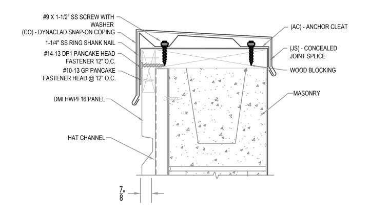
MAXIMUM PANEL ATTACHMENT FASTENER SPACING IS 24" O.C. ALL FASTENERS TO PENETRATE WOOD 3/4" MIN. AND METAL FRAMING 1/2" MIN.
