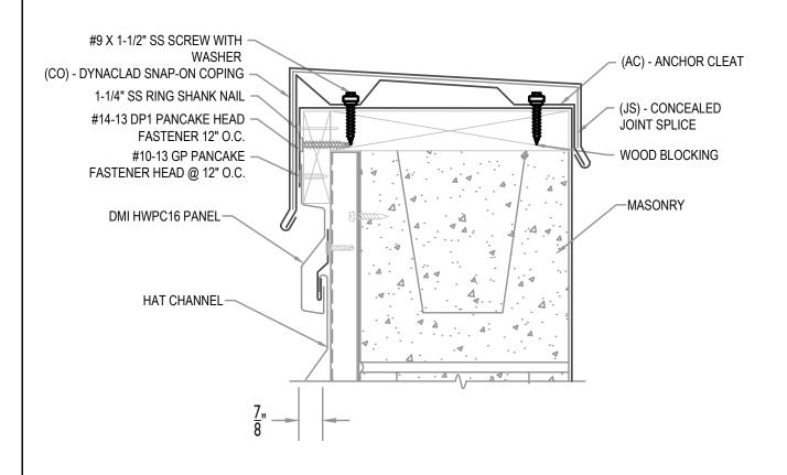
MAXIMUM PANEL ATTACHMENT FASTENER SPACING IS 24" O.C. ALL FASTENERS TO PENETRATE WOOD 3/4" MIN. AND METAL FRAMING 1/2" MIN.
