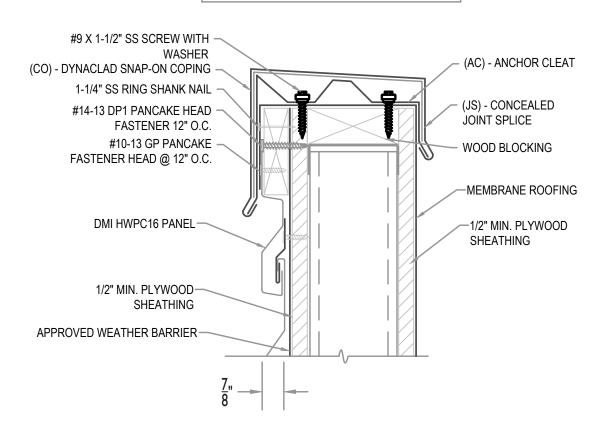
MAXIMUM PANEL ATTACHMENT FASTENER SPACING IS 24" O.C. ALL FASTENERS TO PENETRATE WOOD 3/4" MIN. AND METAL FRAMING 1/2" MIN.
