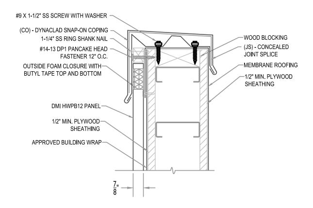
MAXIMUM PANEL ATTACHMENT FASTENER SPACING IS 24" O.C. ALL FASTENERS TO PENETRATE WOOD 3/4" MIN. AND METAL FRAMING 1/2" MIN.
