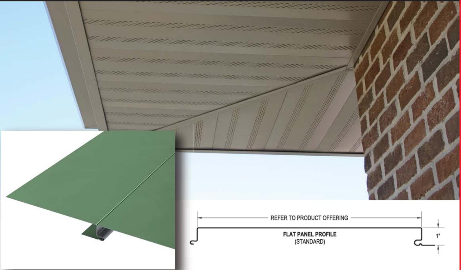
**FLUSH-PANEL FP10** is a commercial grade soffit panel system that provides a flush, aesthetic appearance upon installation. The product is an integral interlocking system by design which installs in one direction from a given starting point.
