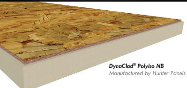
**DYNACLAD® POLYISO NB** is a rigid roof insulation composite panel composed of a closed cell polyisocyanurate foam core manufactured on-line to a fiber reinforced facer on one side and 5/8" oriented strand board (OSB) on the other. DynaClad® Polyiso NB can also be manufactured off-line bonded to 5/8" or 3/4" plywood.
