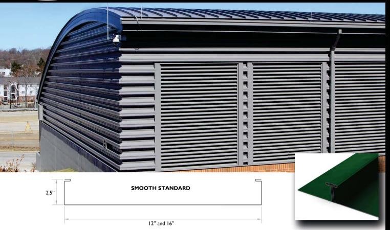
**CURVED TEE-LOCK** (CR-TL25) is a structural panel which is mechanically seamed during installation. The panel is a non-directional system by design which installs in two directions from a given starting point. TEE-LOCK provides installers more control during installation over seam layout and allows symmetry of the panel area. The one piece clip allows for unlimited expansion and contraction.
