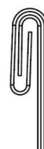
This seam type is commonly referred to as a 180° seam by the additional 90° of travel that the material moved from the 90° profile.
