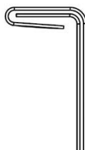
This seam type is commonly referred to as a 90° seam by the 90° of travel that the material moved from the unseamed profile.
