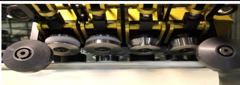
Progressive die rollers positioned over a flat formed section of a roof panel. The panel shows how the rollers bend the metal in each stage to form the desired finished seam.
