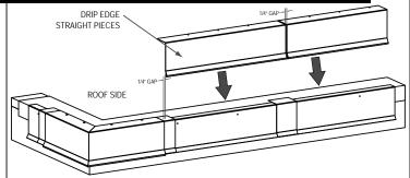
Install drip edge by engaging hem on cleat and rotating back onto roof over membrane. Secure with 1-1/2" stainless steel nails (provided) in all pre-punched holes (6" o.c.). A splice plate is required at every joint. Allow a ¼" gap between drip edge pieces to allow for thermal expansion. Evaluate over-all length of wall before making cuts to ensure proper aesthetics. Minimum drip edg piece length is 24".
