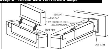
Apply butyl sealant to concealed face of end term as shown. Once sealant is applied install end term and end cap by engaging hem on cleat and rotating back onto roof. Ensure that the end term/end cap abuts wall end. Slide splice plate into end cap/end term until approximately half of the splice plate is left exposed. Secure with 1-1/2" stainless steel nails (provided) into all pre-punched holes (6" o.c.).
