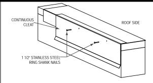
Install continuous cleat by placing top flange of cleat on roof edge over membrane. Once cleat is square with wall install 1-1/2" stainless steel ring shank nails (provided) in all pre-punched holes (12" o.c.). Face heights greater than 6" require a second row of fasteners. Set cleat 2" from all wall ends and miter cleat at corners as required to maintain a continuous cleat line. Abut cleats end to end.
